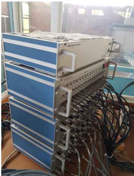
Data Acquisition Deck DHI Collects and shows the wave gauge readings simultaneously
