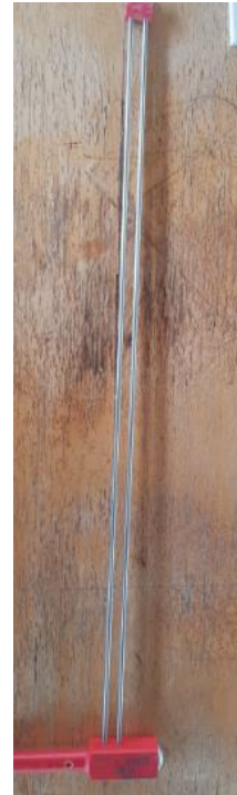
Wave Gauge DHI - TYPE 202 – 60 cm Measures the water surface elevation by measuring the gauge voltages
