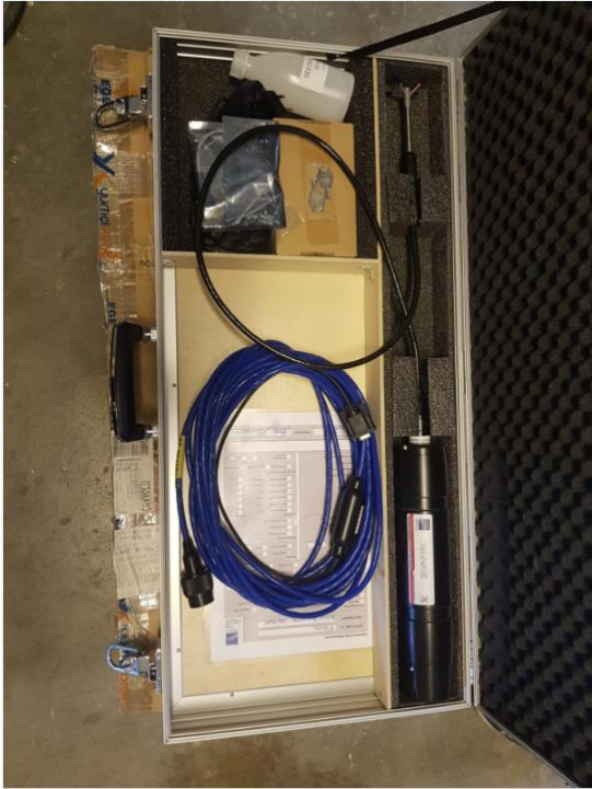
Acoustic Doppler Velocimetry NORTEK AS - VECTRINO+ (PLUS) Measures the instantaneous velocity components of a flow at a single point
