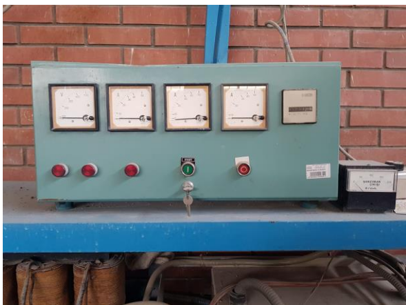
Regular Wave Generator Controller Controls the generation of the regular waves
