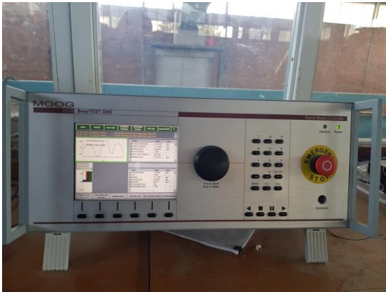
Standard Alone Controller MOOG – SmarTEST ONE Controls the random wave generator
