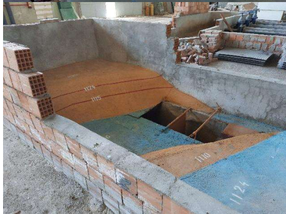
Hydraulic Model of Upper Kaleköy Dam Spillway Experimental setup for investigating optimal spillway design.
