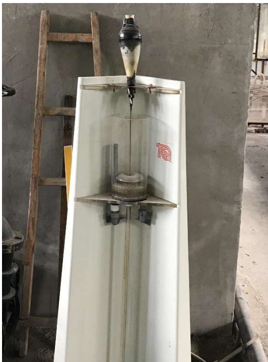
Osborne Reynold's Apparatus Demonstrates laminar flow, turbulent flow and transition between those two.
