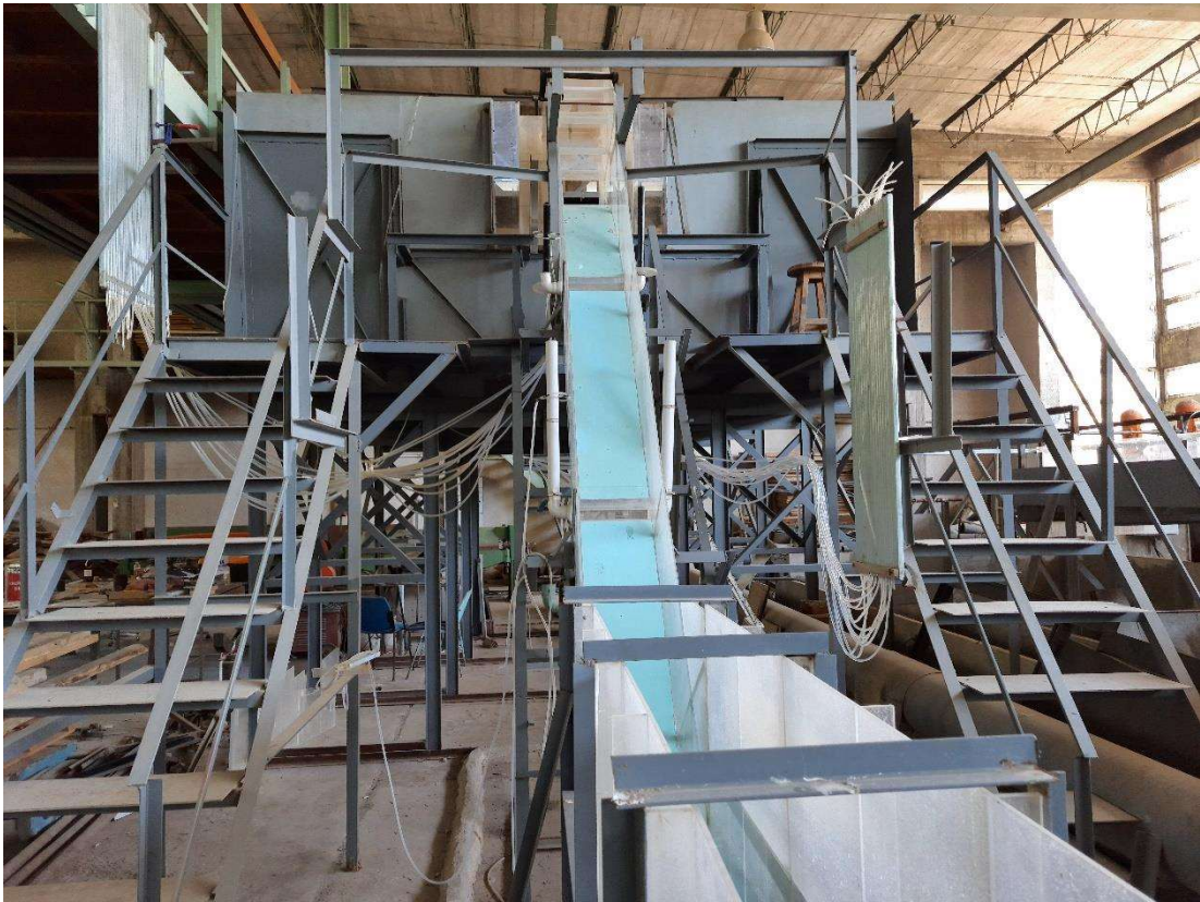
Hydraulic Model of Lower Kaleköy Dam Experimental setup for investigating optimal spillway design.
