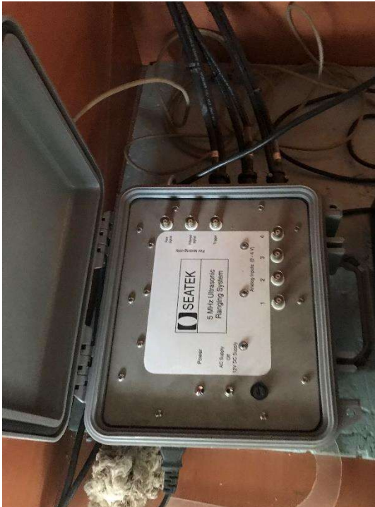
Ultrasonic Ranging System 3-D bed profile measurement device.
