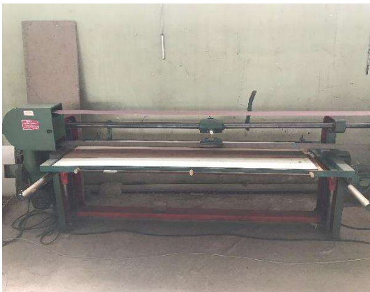
Belt Sander Machine Used in workshop.
