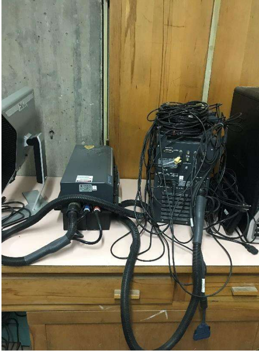
Laser Doppler Velocimetry (LDV) Measures the velocity of semi-transparent fluids using Doppler shift of laser.
