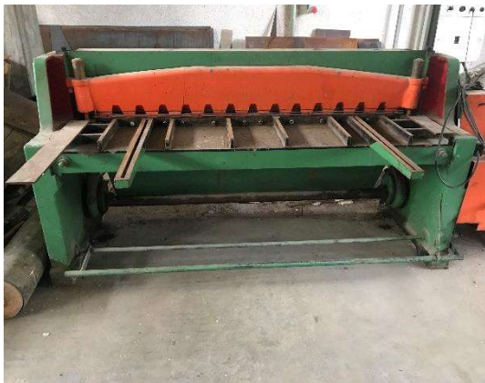
Metal Plate Cutting Machine Used in workshop.
