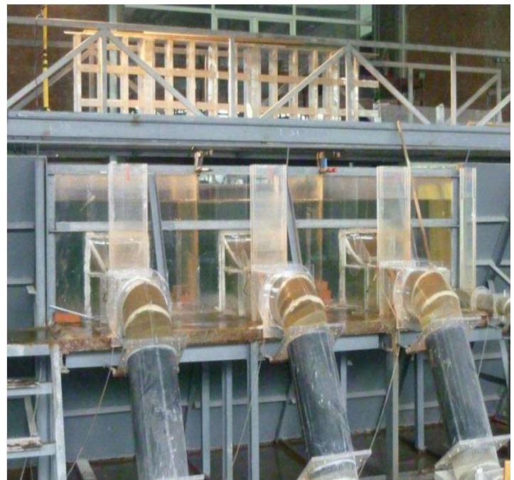
Hydraulic Model of Beyhan 1 Dam (Triple Water Intake Structure) Experimental setup for investigating critical submergence at multiple intake structures.
