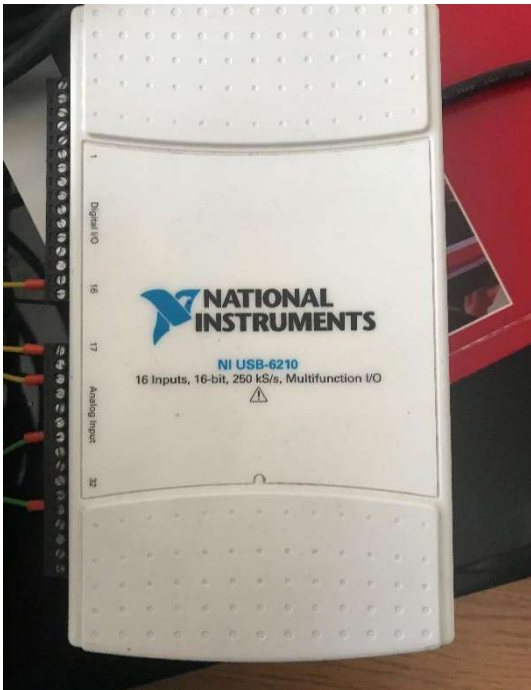
Multifunction I/O Device Multifunction input-output terminal for multiple sensors.
