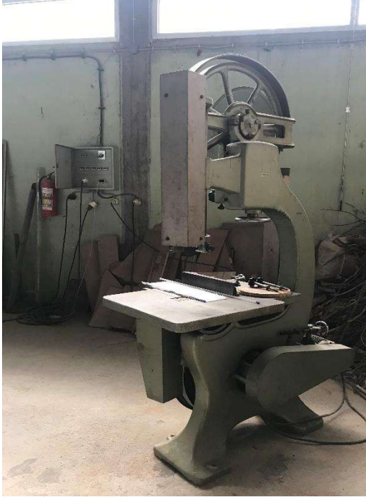
Vertical Band Saw Machine Used in workshop.
