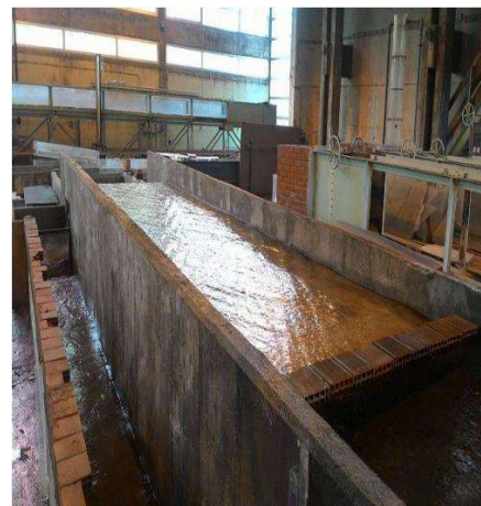
Tyrolean Water Intake Model Experimental setup for investigating optimal design of the Tyrolean water intakes.
