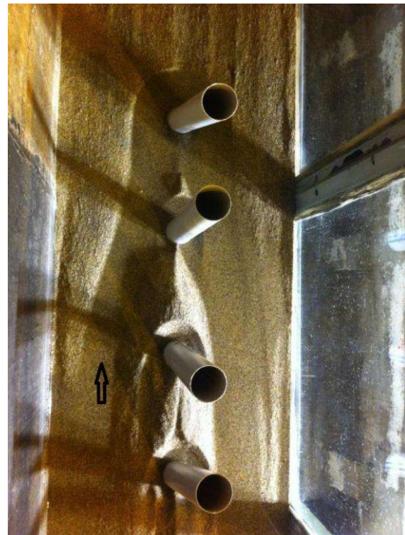
Sediment Channel for Studying Scour Around Vertical and Inclined Piers Experimental setup for investigating local scours around bridge piers.
