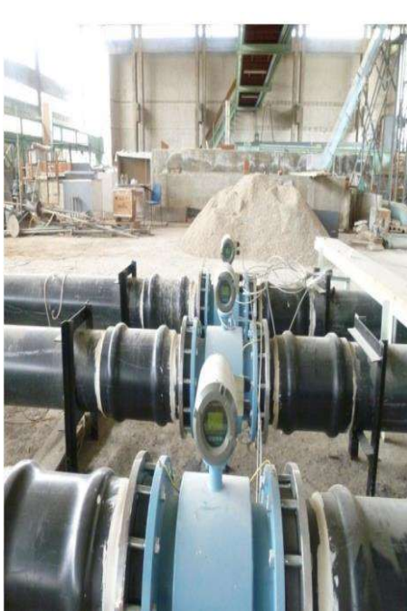
Hydraulic Model of Beyhan 1 Dam (Triple Water Intake Structure) Experimental setup for investigating critical submergence at multiple intake structures.
