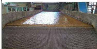
Tyrolean Water Intake Model Experimental setup for investigating optimal design of the Tyrolean water intakes.
