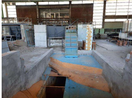
Hydraulic Model of Upper Kaleköy Dam Spillway Experimental setup for investigating optimal spillway design.
