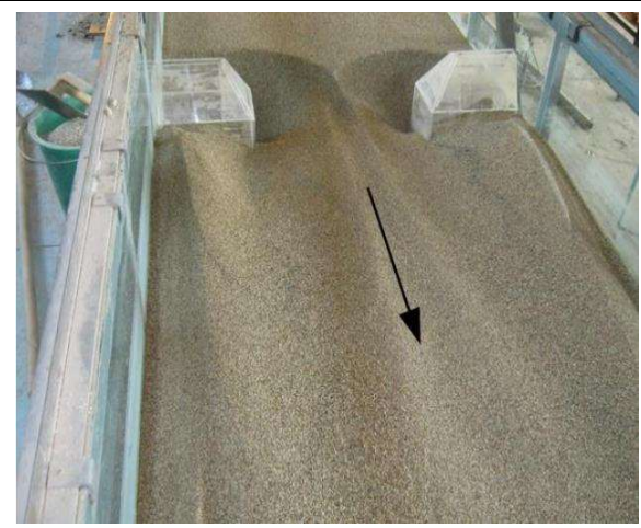
Fixed Slope Open Channel (Sediment Channel) Experimental setup for investigating local scours around bridge elements.
