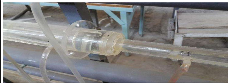
Apparatus for Head Losses Through Single and Parallel Pipes with/without Expansion and Contraction of Pipe Diameters Laboratory setup for Hydromechanics course (CE372).
