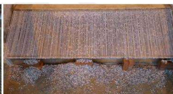
Tyrolean Water Intake Model Experimental setup for investigating optimal design of the Tyrolean water intakes.
