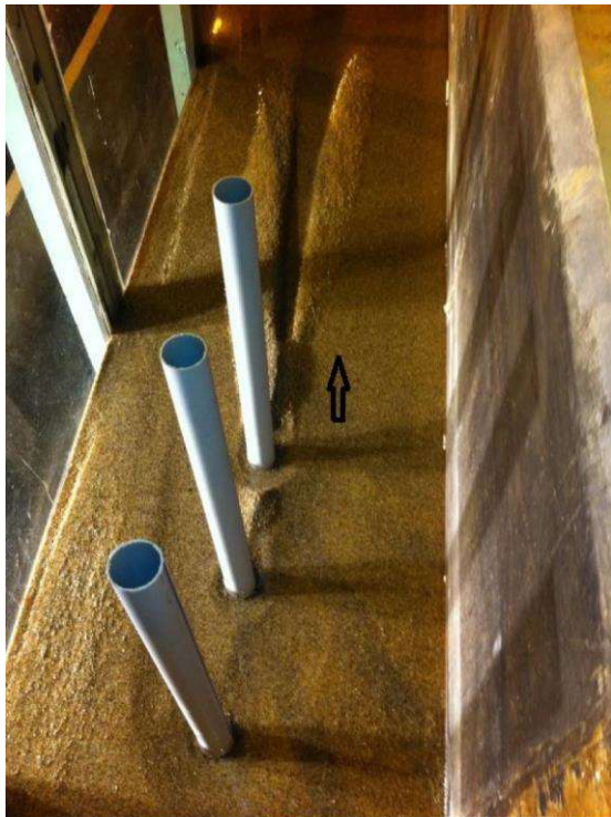
Sediment Channel for Studying Scour Around Vertical and Inclined Piers Experimental setup for investigating local scours around bridge piers.
