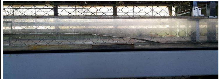
Open Channel Test Apparatus Laboratory setup for Hydromechanics course (CE372). Transitions and Hydraulic Jump phenomenon are demonstrated in the open channels
