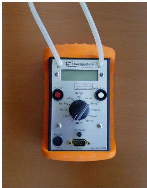
Digital Manometer, Air Speed Meter and Air Flow meter Measures the air flow.
