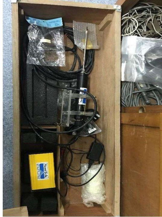
Acoustic Doppler Velocimeter (ADV) Measures the velocity of fluids using Doppler shift of sound waves.
