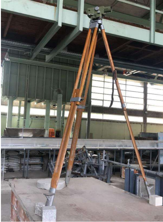
Levelling Instrument (Nivo) Optical leveling instrument.
