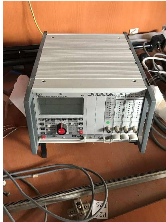
Data Acquisition Equipment Monitors, amplifies and records analog signals from multiple sensors.
