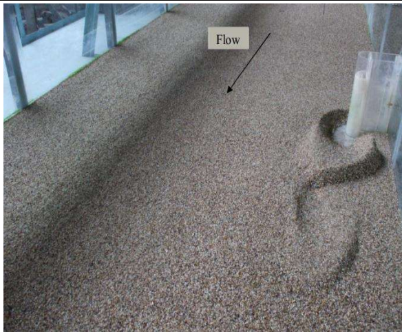
Fixed Slope Open Channel (Sediment Channel) Experimental setup for investigating local scours around bridge elements.
