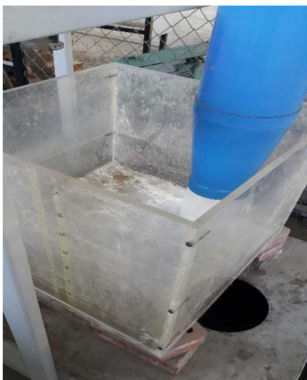
Open Channel Test Apparatus Laboratory setup for Hydromechanics course (CE372). Transitions and Hydraulic Jump phenomenon are demonstrated in the open channels
