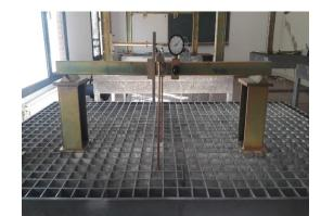
Lab4: Flexural (Bending) Deformation
